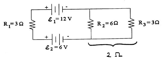
a. Calculate the voltage across resistor  $R_1$ . (10 pts.)
