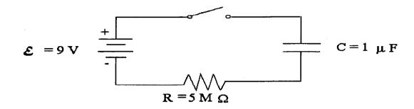
a. What is the current in the resistor just after the switch is closed? (5 pts.)
