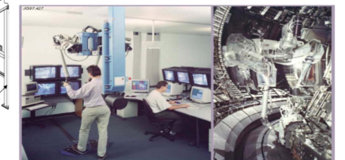
Figure 3.4.2: MASCOT Manipulator - Master (left) and Slave (right)
